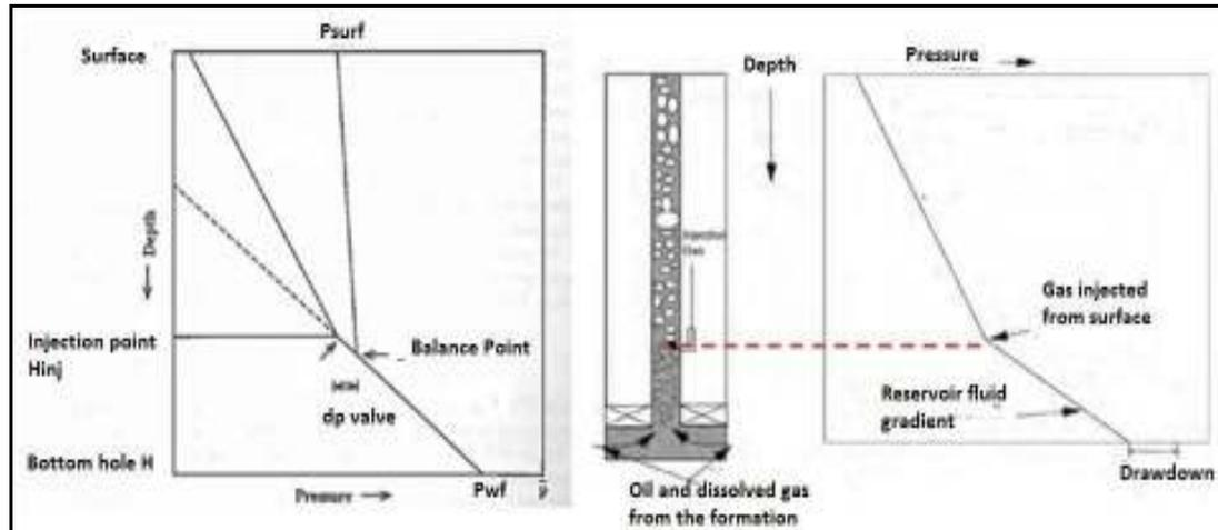
**Figure (2.2) Single-injection gas lift installation (Fathi Elldakli, 2017)**
