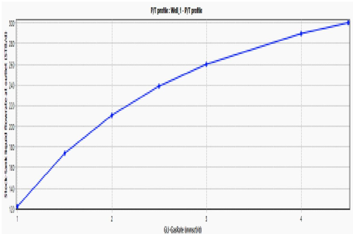
**Fig (4.3) GLI-Gas Rate vs. Liquid flow rate**
