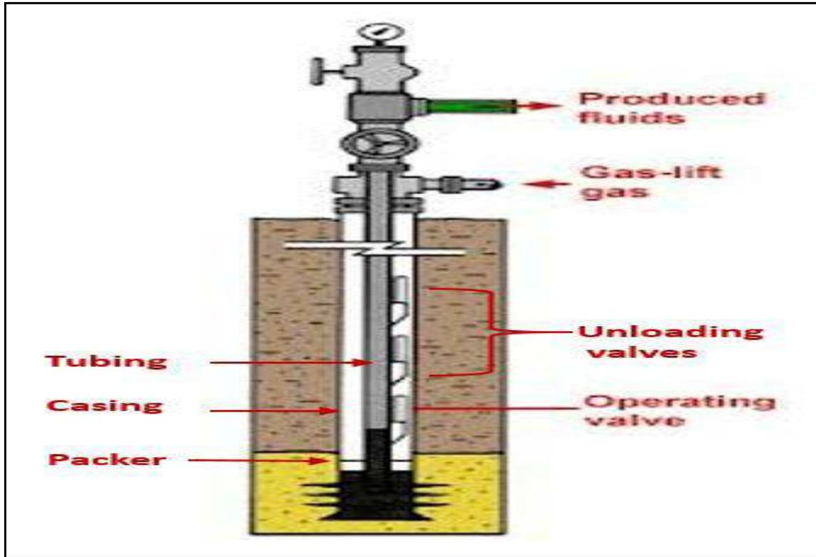
**Figure (2.3) Well with multiple GLV at different depths (Fathi Elldakli, 2017)**
