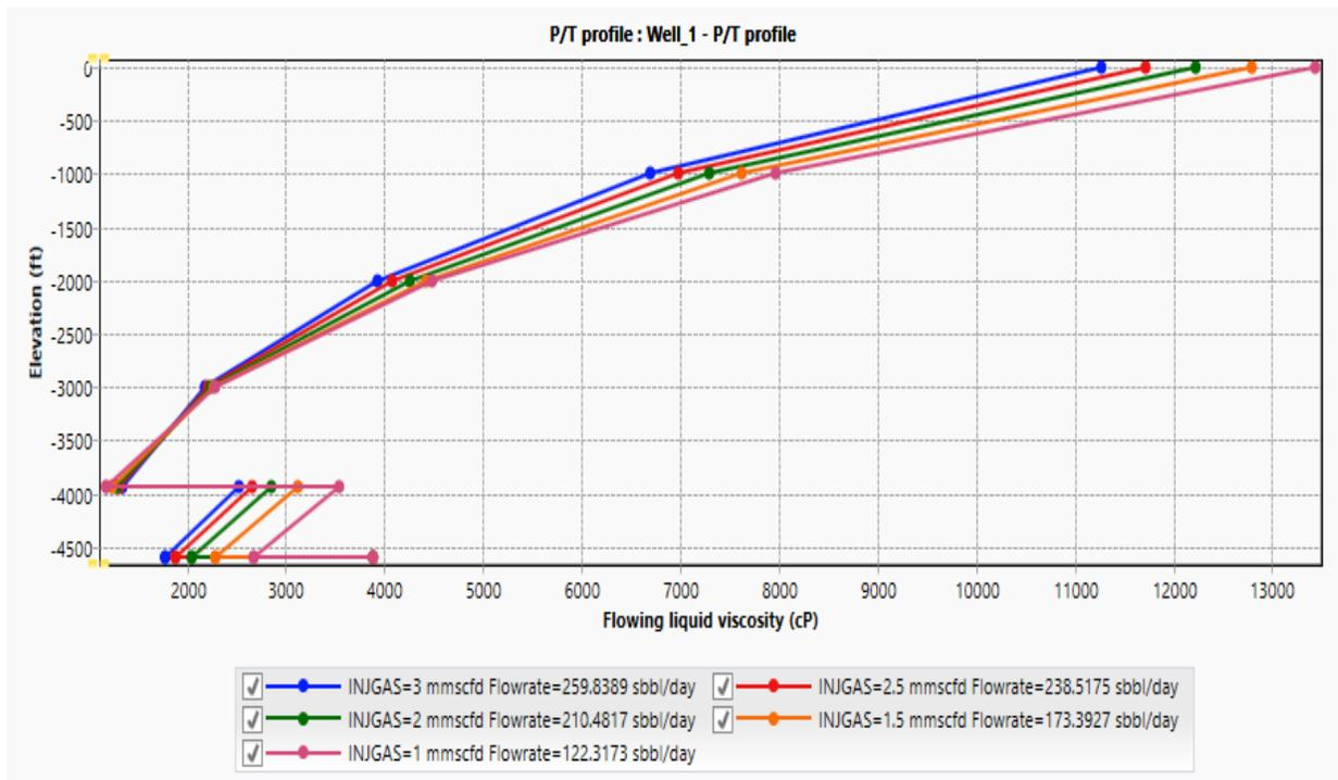
figure (4.1) Liquid flowing viscosity
