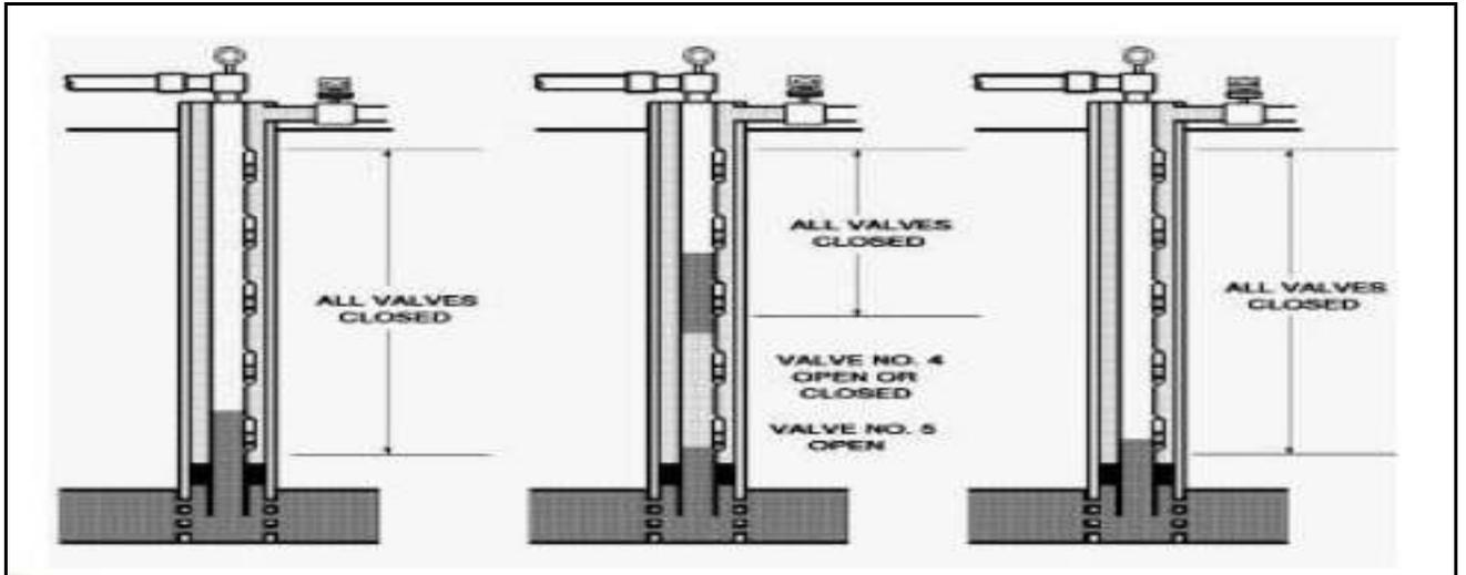
Fig (2.7) intermediate gas lift (Brown KE, 1984).
