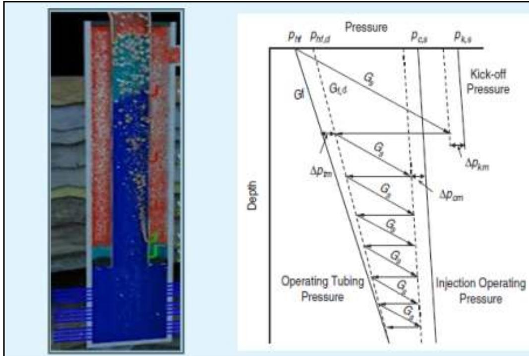
**Figure (2.4) String design for GL system and the depth of the valves
