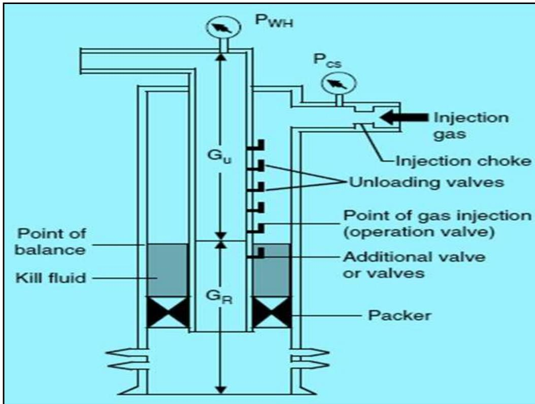
**Fig(2.6) continuous gas lift**
