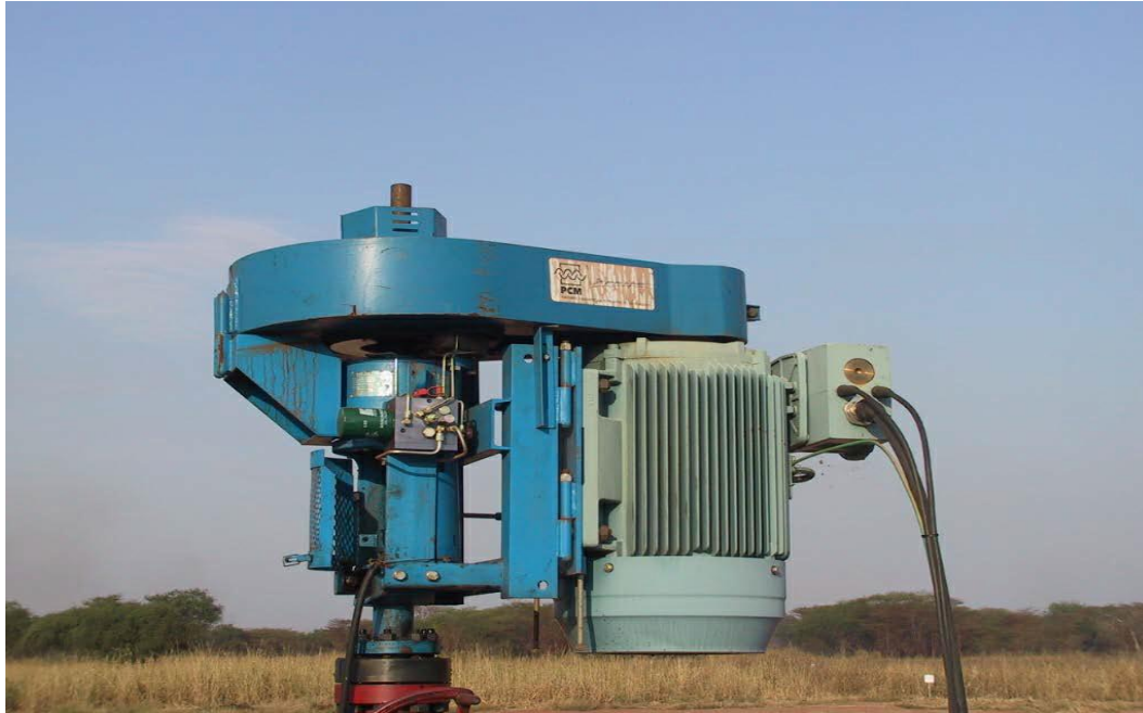
Figure (2.2) Basic surface equipment for PC pumping systems (Larry, 2006)
