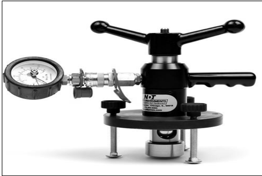
Fig. (2.6): A typical setup of pull-out resistance NDT methods (Adapted from http://www.ndtjames.com ).
