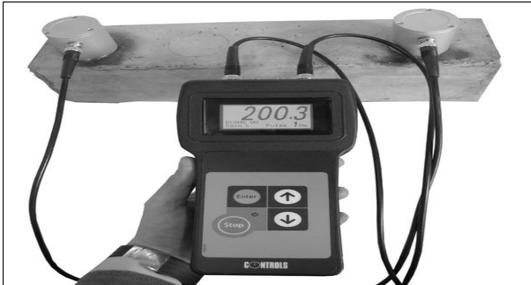
Fig.(2.10): Ultrasonic pulse velocity test apparatus(Adapted from http://www.controls-group.com ).
