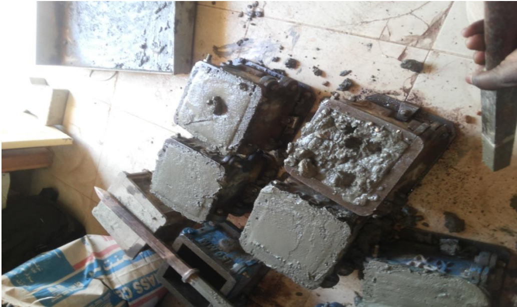
Image 2: Concrete Cubes Finishing
