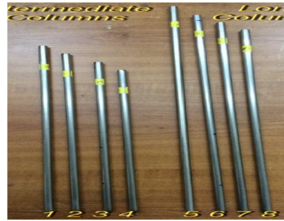
Figure 1: Buckling specimen for long and intermediate columns.
