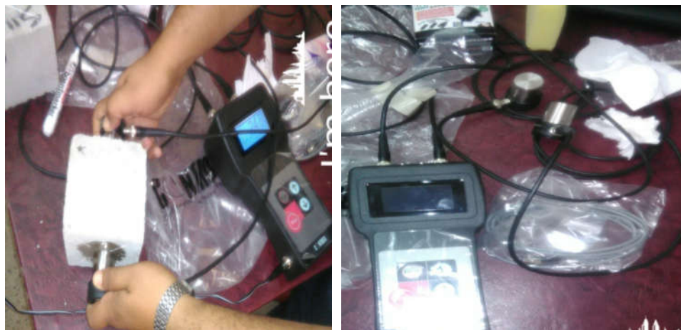
Fig 3.10 ultrasonic pulse test, direct transmission
