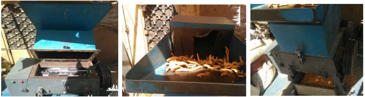
Fig3.3 Specimens preparation by hredder/crusher machine for industrial EVA waste
