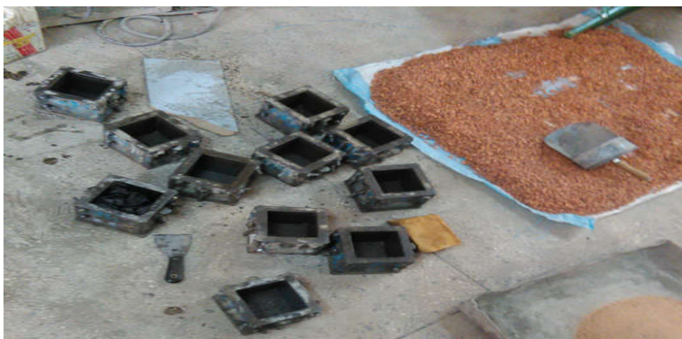
■ Fig 3.5 Cubse test for concrete mixes BS1881
