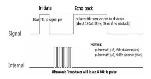
Figure 3.6: Ultrasonic Trigger and echo pulse
