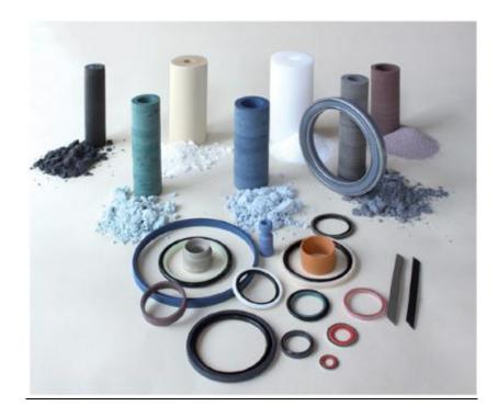
Figure 3.8: PTFE powder, semi-finished shape and final machined product [23]
