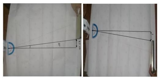
(a) Left side (b) Right side Figure 4.7: Detection zone at specific distance and angle
