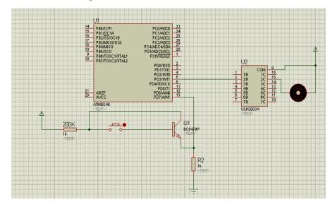
Figure 3.9: water detector circuit
