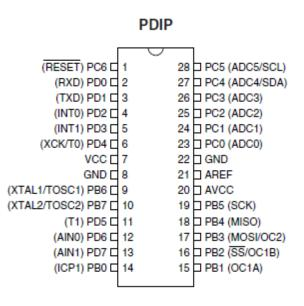
Figure 3.4: AT mega 8l pin configurations
