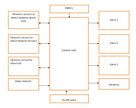
Figure 3.1: Block diagram of the interactive cane
