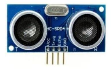
Figure 3.5: HC-SRO4 ultrasonic sensor.
