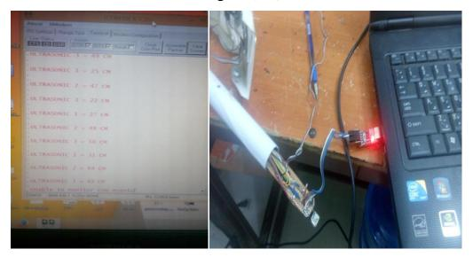
Figure 4.5:HCSR04 sensor distance test
