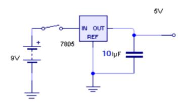
**Figure 3.7: The power stage of interactive cane**
