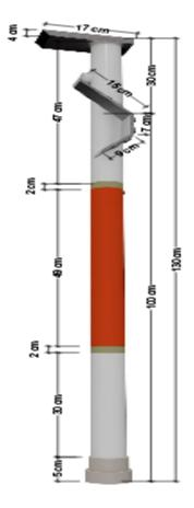
Figure 4.1: Dimension of guide cane
