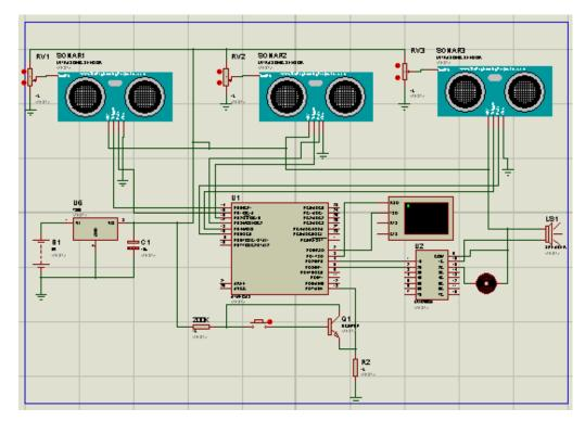
Figure 3.3: The whole circuit design using proteus simulation.
