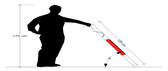
Figure 4.3: Side elevation of guide cane and height of blind person.
