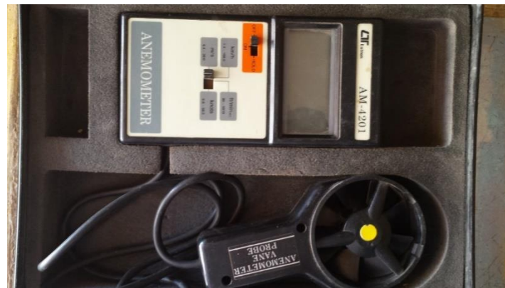
Figure [3.7]: The anemometer
