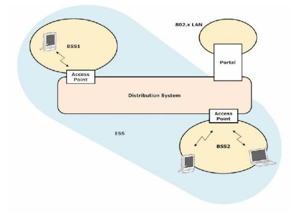
Figure 2-3: WLAN Infrastructure based architecture
