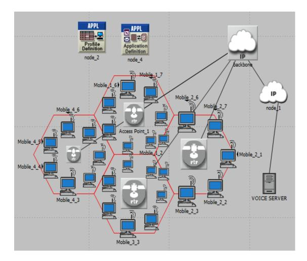
Figure 3-4: WLAN network topology
