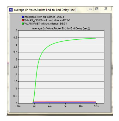
Figure 4-14: average packet end to end delay without silence suppression
