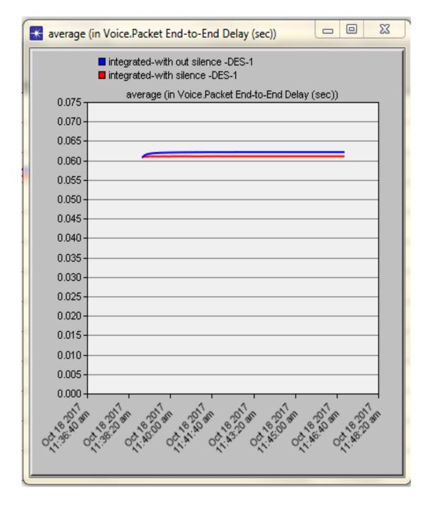
Figure 4-9: Integrated network average end to end delay
