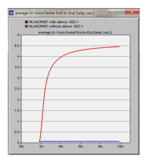
Figure 4-6: WLAN packet end to end delay
