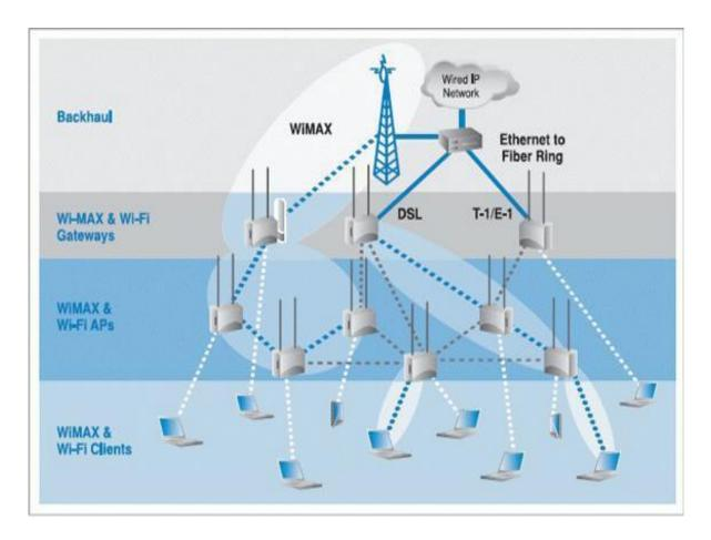
Figure 2-6: Wi-Fi –WiMAX Fully Integrated Architecture
