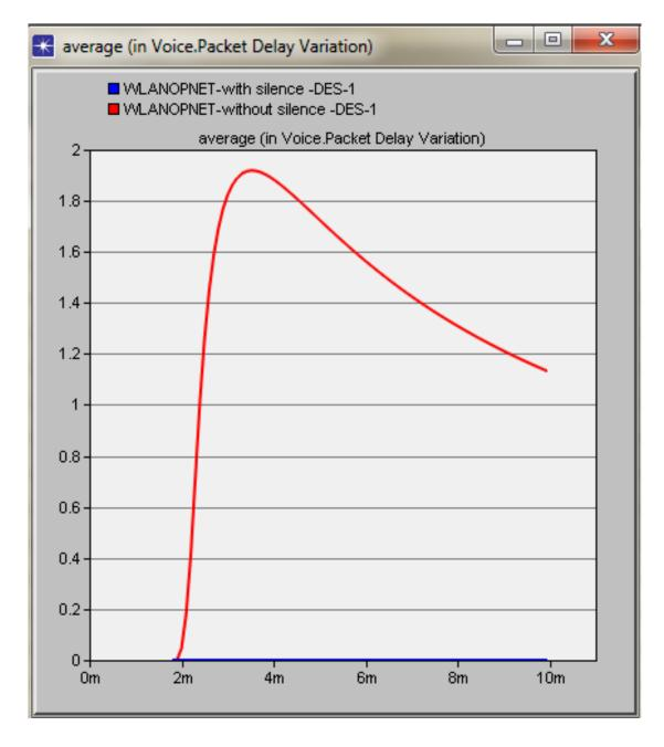
Figure 4-5: WLAN average packet delay variation
