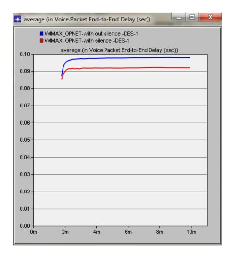
Figure 4-3: WiMAX packet end to end delay
