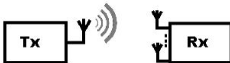
Figure 2.3: SIMO : Single input Multi output.
