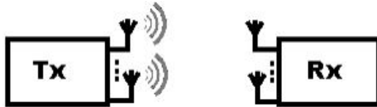
Figure 2.5: MIMO : Multi input Multi output.
