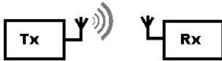
Figure 2.2: SISO : Single input single output.
