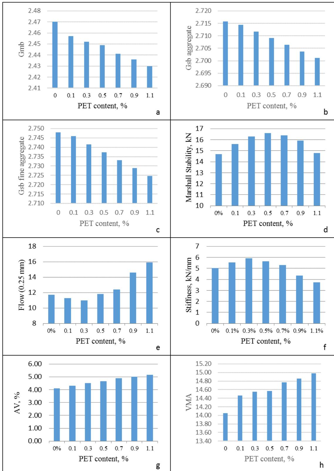
Figure 2: Results of Marshall tests
