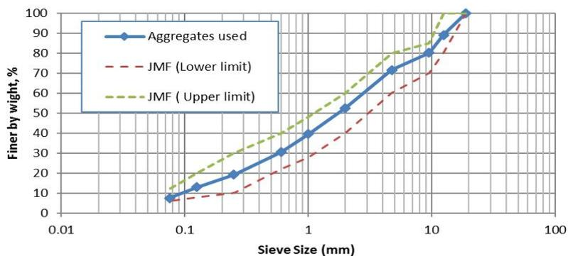
**Figure 1: Aggregate gradation**
