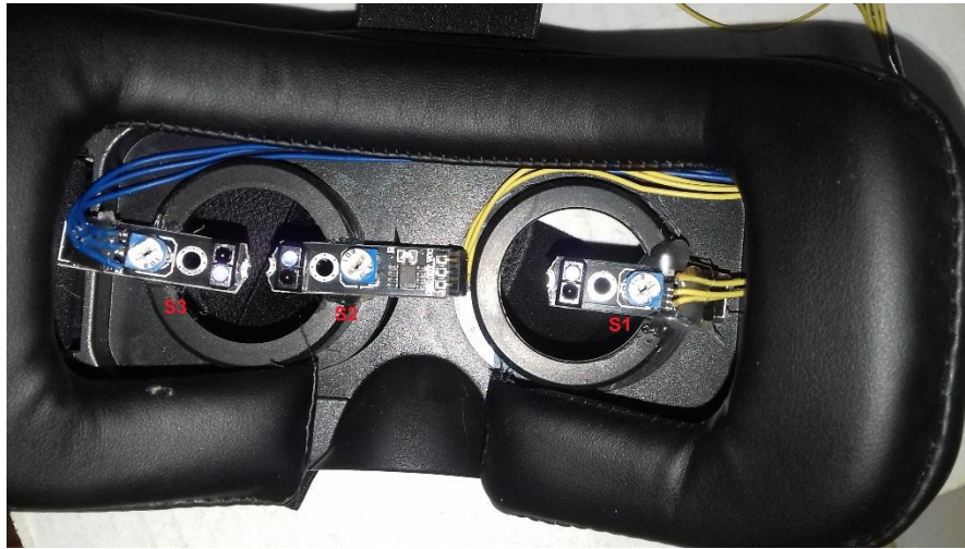
Figure 3. 6 Sensors Positioning on the Frame
