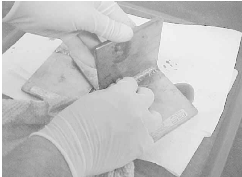
Figure (4-5) Removal of excess surface penetrant.
