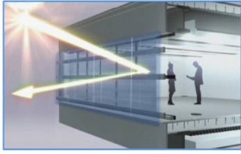
Low E Coating Skin and Blind reflected solar radiation
