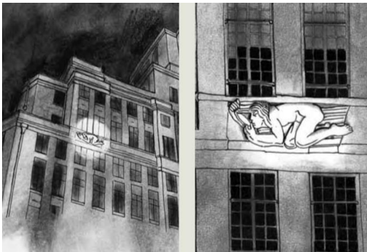
Figure 3.18 lighting selected feature Source: external lighting for historic buildings
