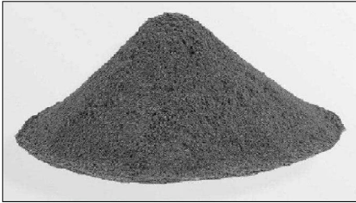
Figure (2.1) As-produced silica fume. This is what the material looks like after it is collected.
