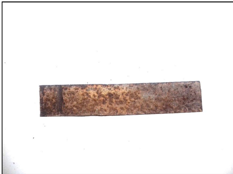
Fig (3-2): sample (a) iron with rust
