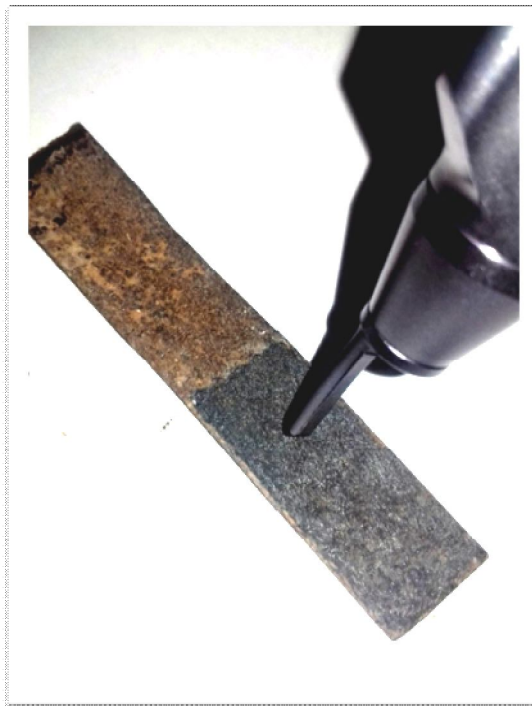
Fig (4-4): Sample (a) after finished particular cleaning
