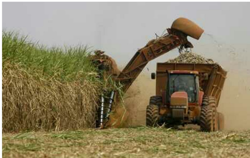
Fig. (1-4b): Harvesting of sugar cane by machine
