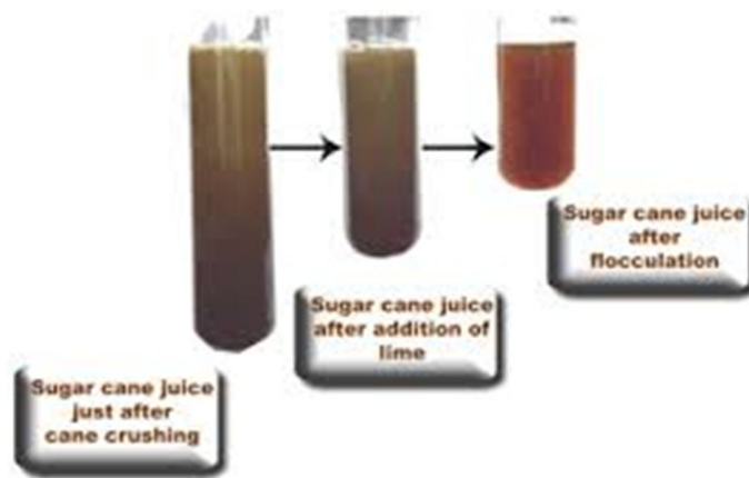
Fig. (1-7a): The juice from the extraction until the end of the clarification
