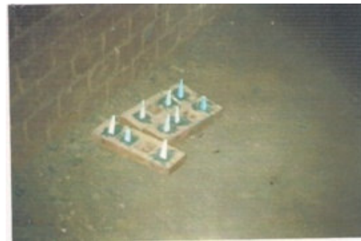
Plate 2 The three groups of seger cone before firing
