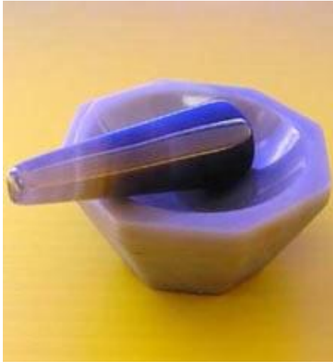
Figure (4.3) Gate mortar
