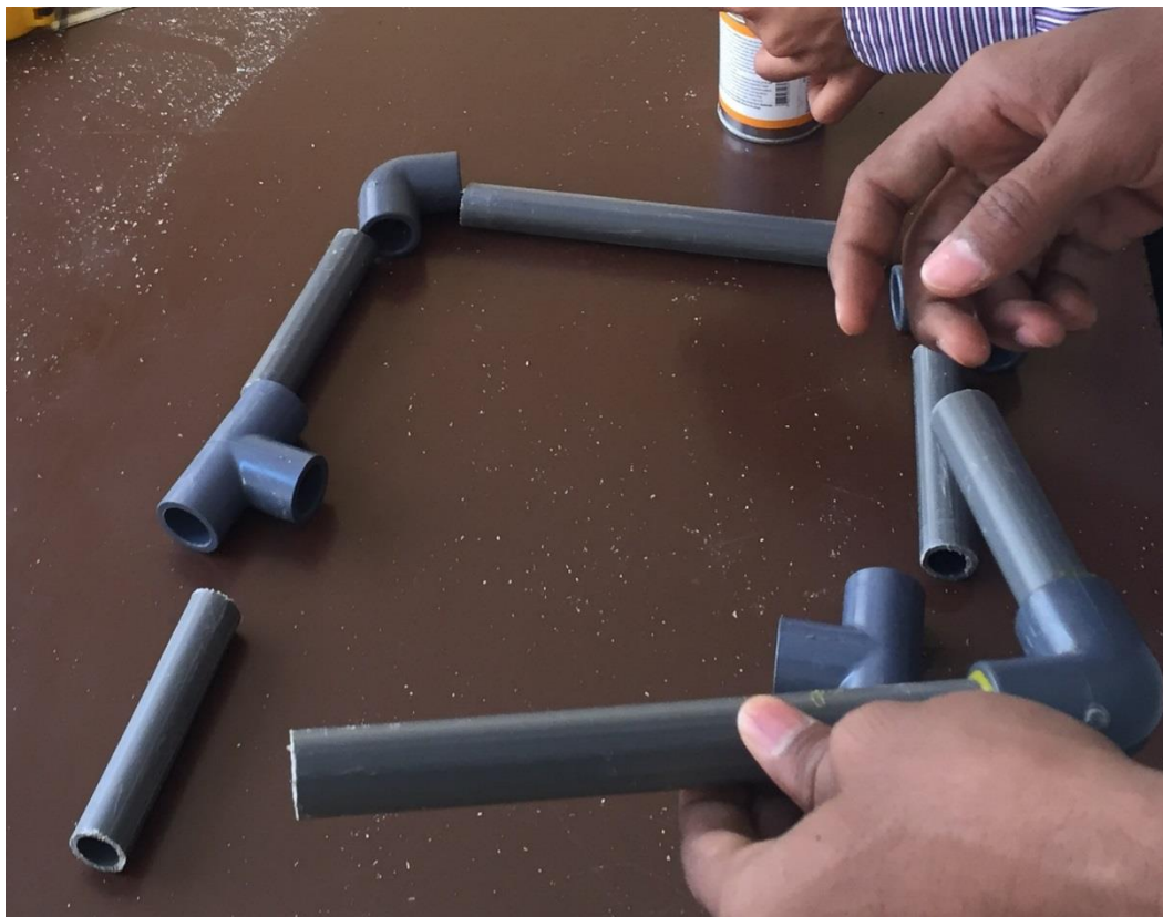
Figure 4.3: Cutting and linking PVC pipes
