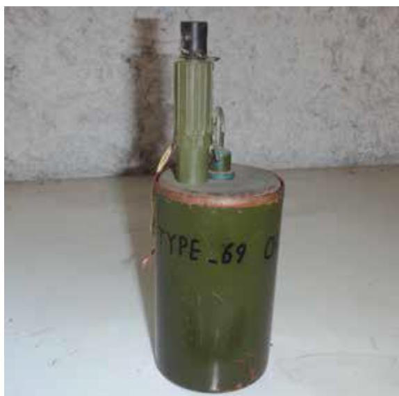
Figure 2.9: Bounding AP mine
