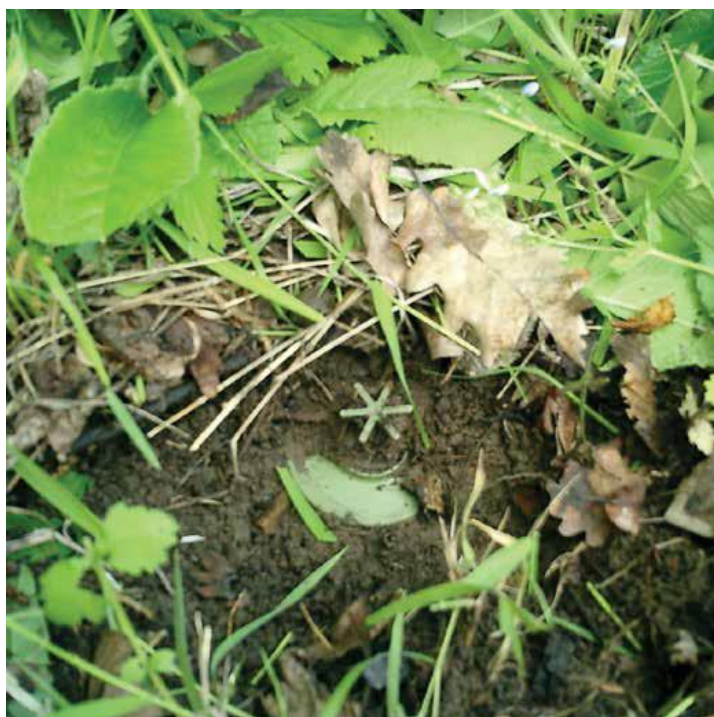
Figure 2.4: metal blast AP mine planted in the ground.
