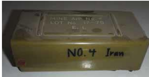
Figure 2.5: plastic blast AP mine.
