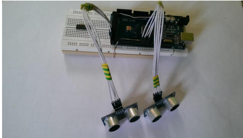
Figure 4.5: the two ultrasonic Connected to the Arduino Mega
