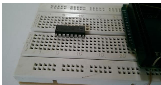
Figure 4.2: Plugging in the motor driver to the breadboard
