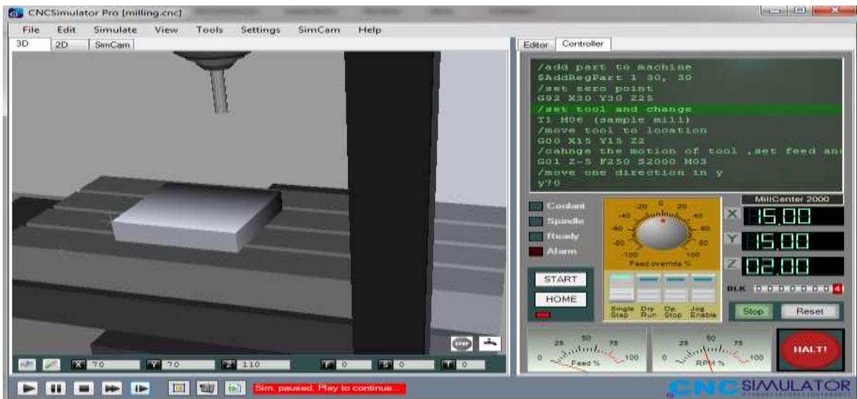
Fig.4.22: Setting the zero point (reference point)
