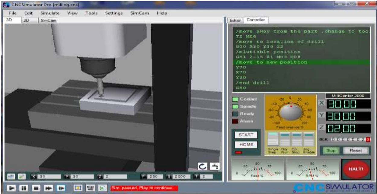
Fig.4.33: Achieving the hole No: 1 (G81 Z-15 R1 M03 M08)
