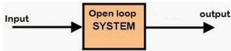
Figure3.1:open loop system
