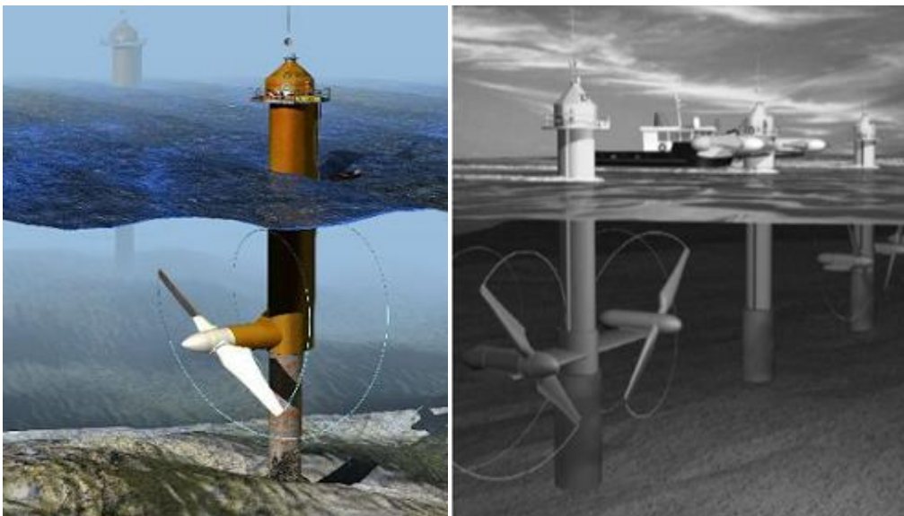
Figure 4.8 : Horizontal axis turbine
