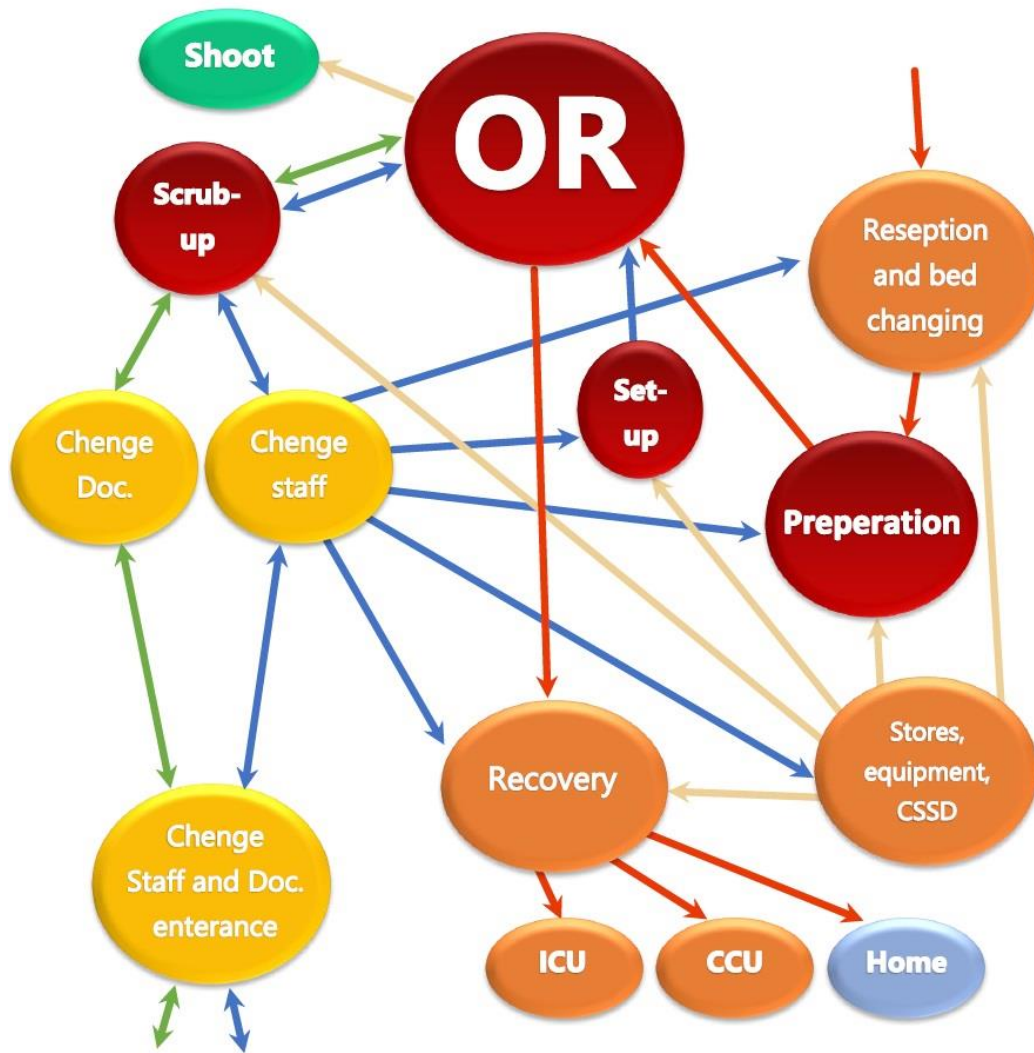
Figure (5.1): flow diagram of human and materials in the operation complex
