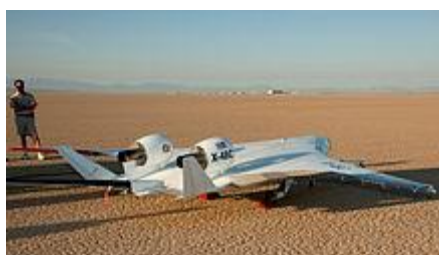
Figure 2.20 The X-48C featuring two engines and inboard vertical stabilizers
