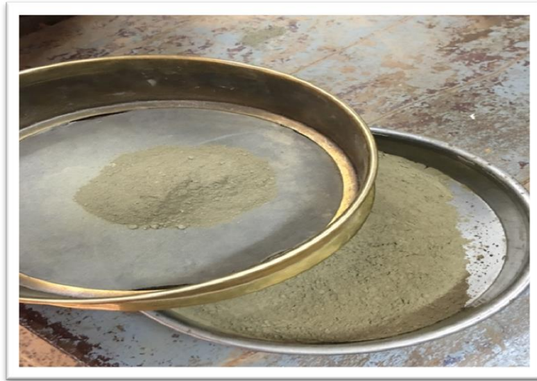
Figure (3.5): Local Bentonite sample sieving by using 75 micron opening mesh. (SUST Lab)
