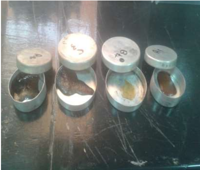
Plate 9- Aluminum Dishes to determine moisture content
