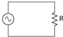
Figure (3.7.1) A purely resistive circuit
