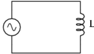
Figure (3.7.2) A purely inductive circuit
