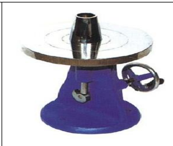
Apparatus for testing for measure Mortar flow
