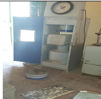
Compressive testing machine
