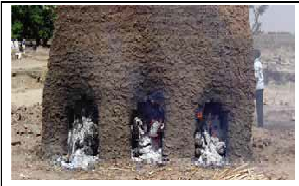
Photo graph 2.9: Brick kiln fired with wood Environmental threats UN-HABITAT (2009).
