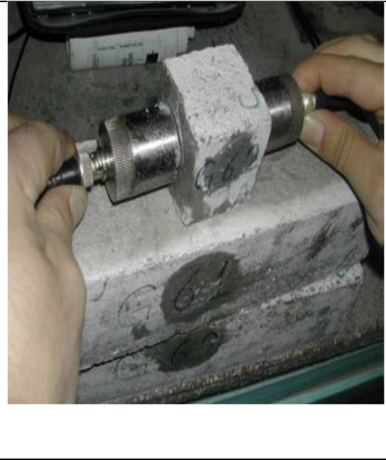
Through cubical specimen UPV test
