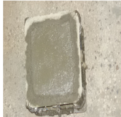
Casted (150x150x150) mm concrete moulds
