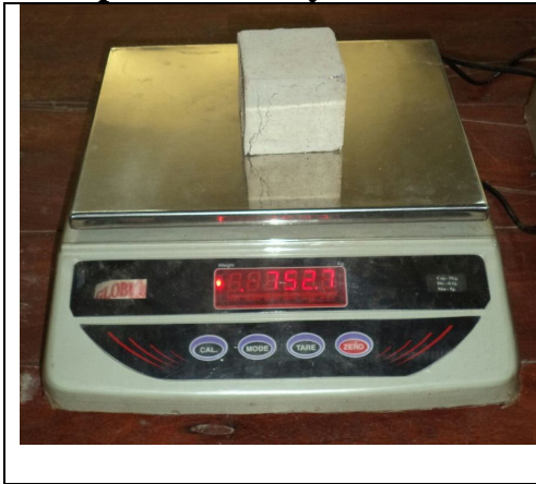
Electric Balance used for weighting samples.
