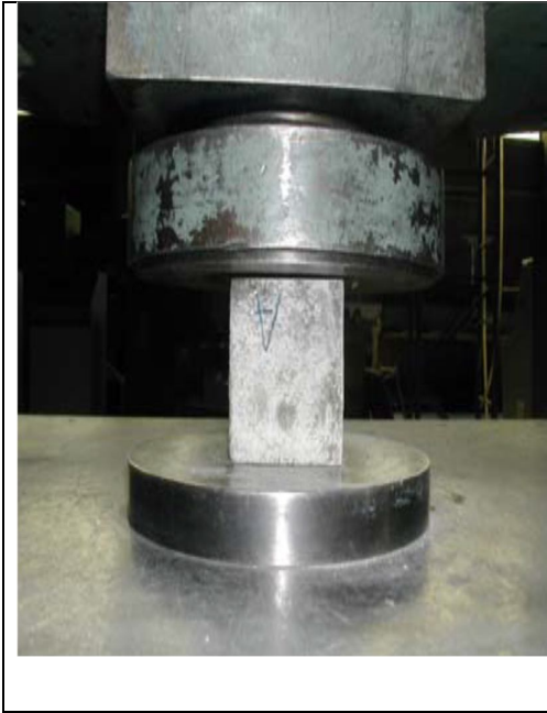
Compressive testing Machine (Mortar cube)
