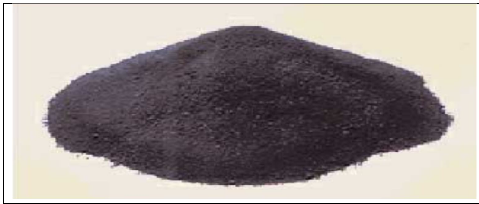
Photo graph 2.6: Silica Fume Powder (Siddique and Khan (2011))
