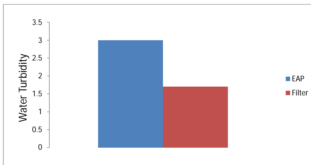
Fig 4.4 Comparison between water turbidity level in Blue Nile water after hydro cyclone filtration and United States Environmental Protection Agency Standard( EAP)
