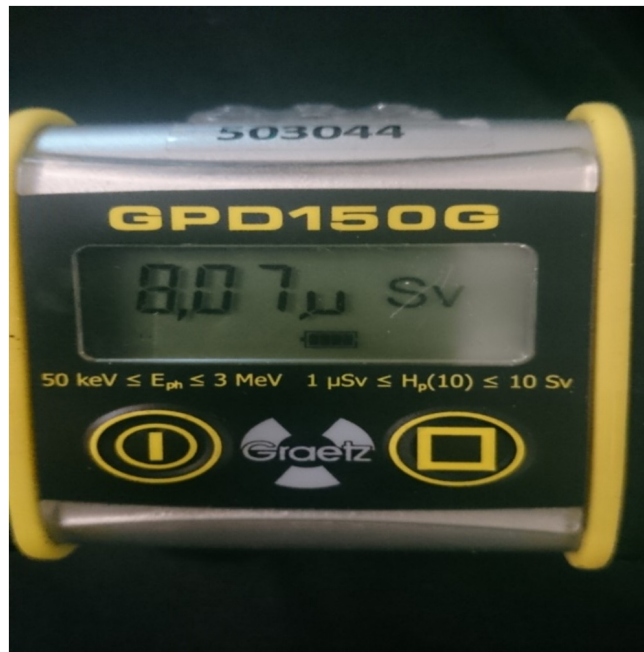
Fig 3.2: digital pocket dosimeter GPD150 product by PTW which used in this study.
