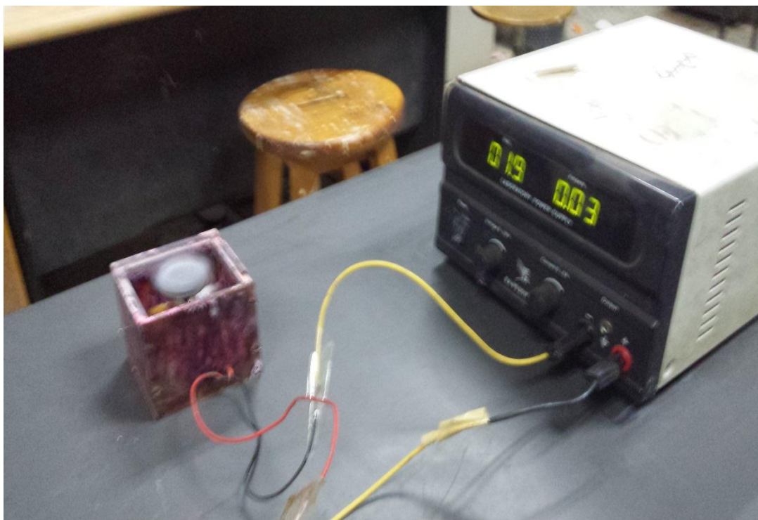
Fig (4-3): Spin Coating for the sample
