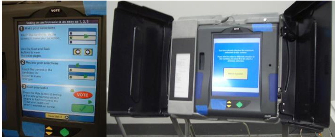
Figure 2.4: Direct Recording Electronic Voting Machine [15]
