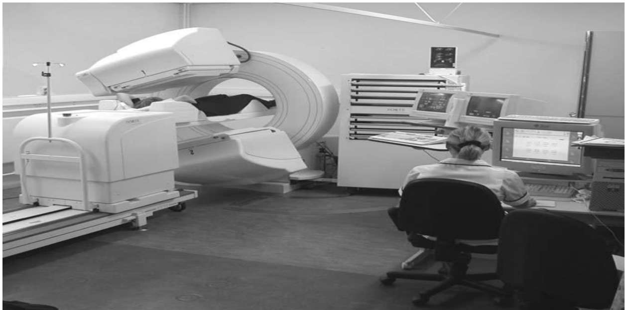
Figure (2.1) The gamma camera. The patient is lying between the detectors of this double-headed system. To the right of the camera is a rack containing extra
