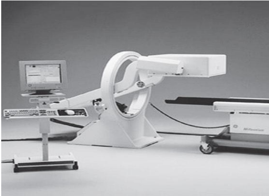
FIGURE (2.5) Single-headed gamma camera mounted on a rotating gantry. The camera is operated from the computer (left). The flexible positioning of the camera head and the bed (right) allows the system to obtain images of many different parts of the body.
