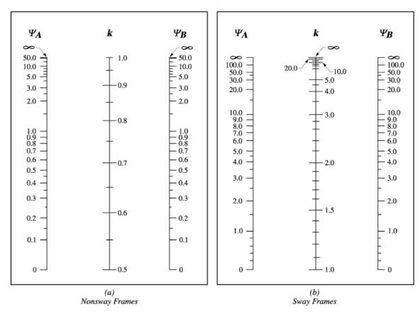
$\Psi$  = ratio of  $\Sigma(EJ/\ell_c)$  of compression members to  $\Sigma(EJ/\ell)$  of flexural members in a plane at one end of a compression member  $\ell$  = span length of flexural member measured center to center of joints
