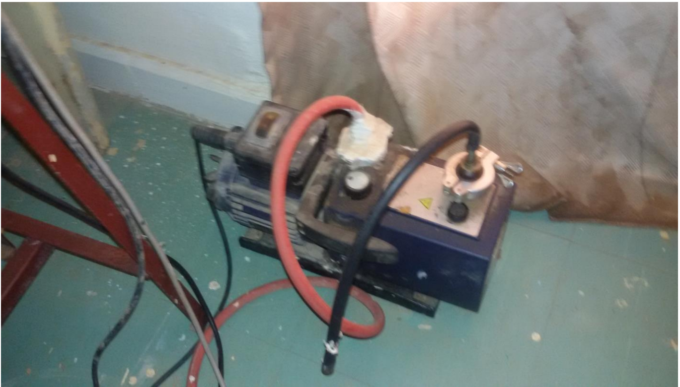
Fig.2.2: Vacuum pump photograph
