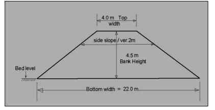
Fig.(5.20):Cross Section Of Outer Guide Bank
