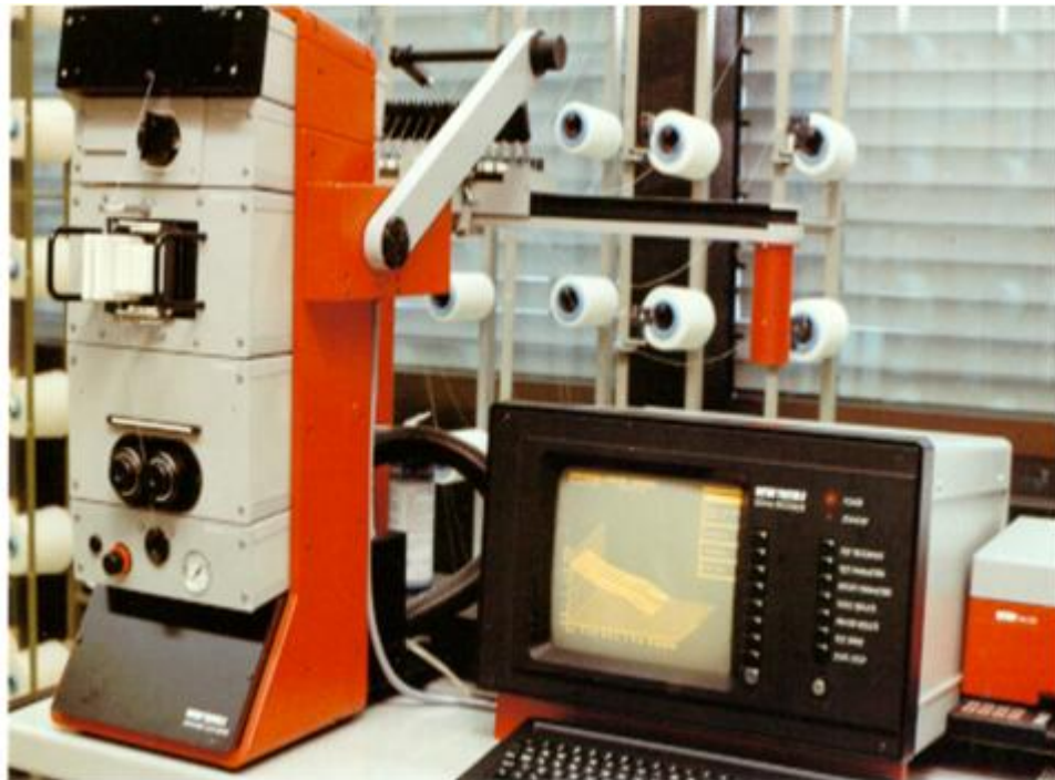
Figure3.1: Aphoto of Uster evenness tester3(Zellweger)
