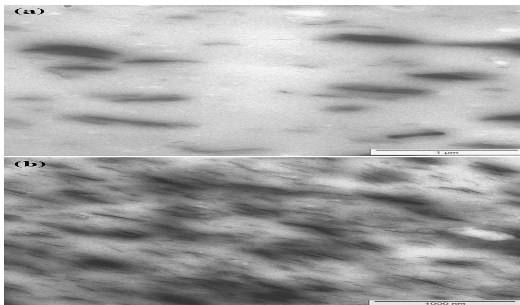
Fig. 5 TEM image at of a NR/2 phr DDA-MMT and b NR/3 phr FAs-MMT
