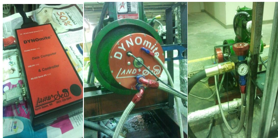
Figure 3.8: Hydraulic Dynameters. And A Personal Computer to Monitor and Control Dynamometer
