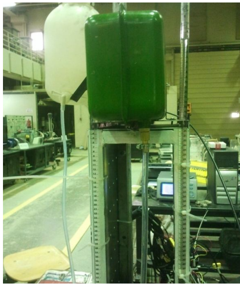
Figure 3.6: Diesel Tank, Burette for Diesel, Ethanol/Water Tank, Burette for Ethanol/Water
