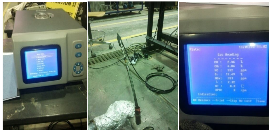
Figure 3.7: Gas Analyzes, Sampling Tube in Exhausts Manifold, Display
