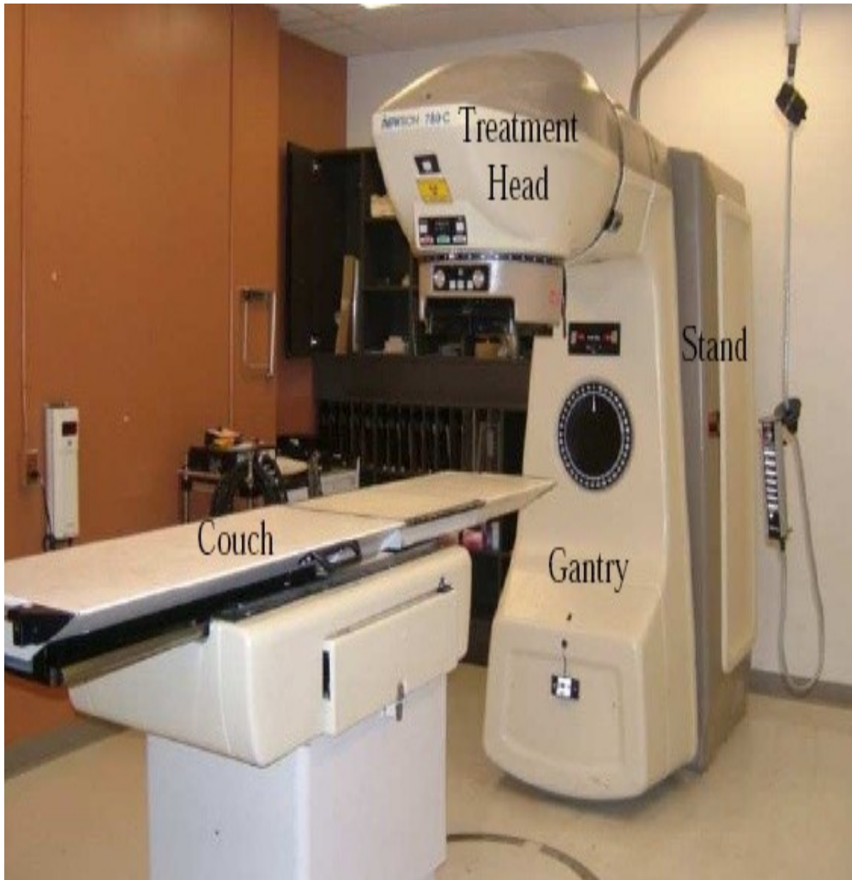
Figure (1.5) Photograph of the Theratron 780C Co-60 Radiotherapy unit, adapted from Joshi et al. (2008).
